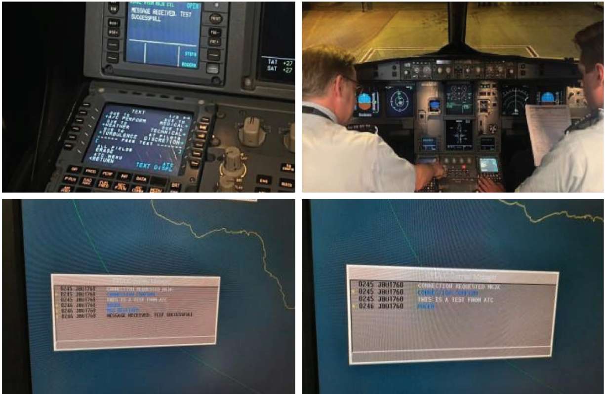
Fig. 3 above shows successful CPDLC testing with JetBlue airlines. Top images feature the Jet Blue aircraft cockpit, while the bottom photos show the Kingston Air Traffic Control Centre (KATCC) equipment room test bed.
